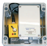
Receiver RBX in protective housing (lid off)
